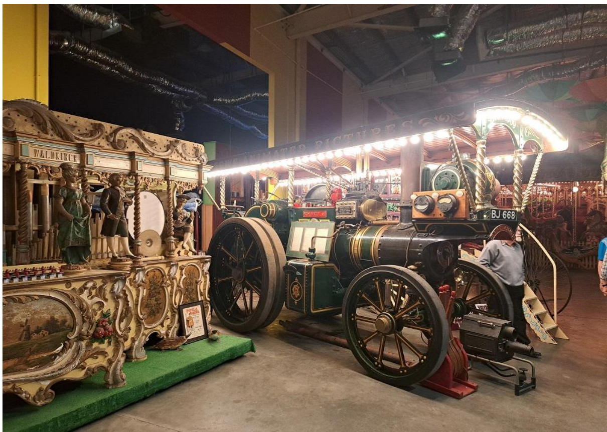
A Showman's engine at Fairground Follies – historically they both towed fairground vehicles and supplied electricity to the fair.
