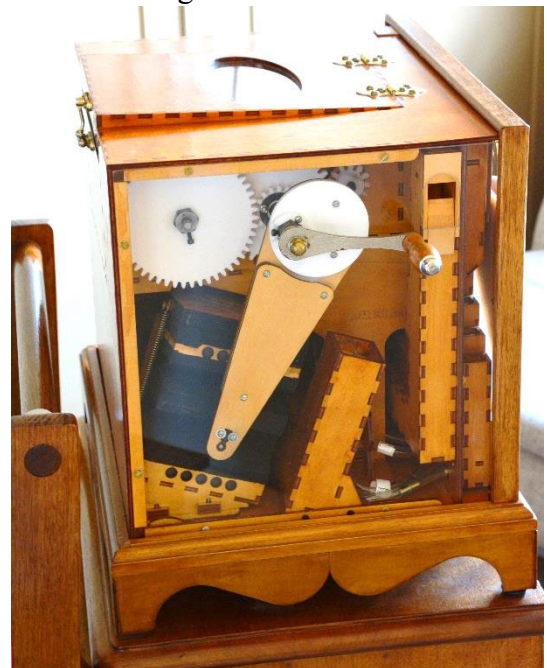
Custom Perspex side panel to show bellows and crank and bass pipes.
